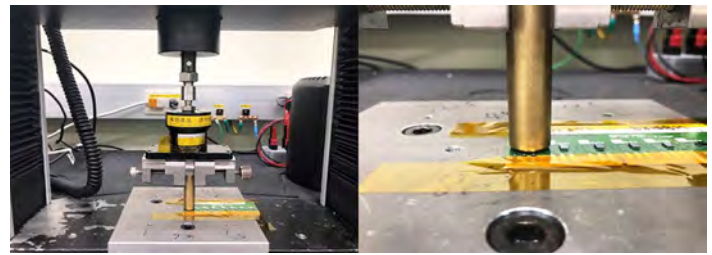
Figure 17: Pressure test instrument. The tester head lowers to the backside of the devices using a constant loading speed of 0.6 mm/min until the predetermined force is sensed by the gauge. The DUTs are surface mounted on a FR4 test coupon that is secured on the testing stage.
